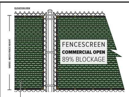
• FENCESCREEN PANELS WITH 2" POLYPROPYLENE WEBBING FOR EDGE REINFORCEMENT.
